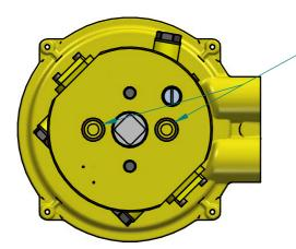
Ensure o-rings are present Double acting - 2 off o-rings Spring return - I off o-ring
