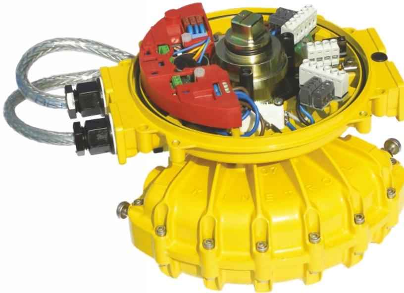
The P3 On/Off positioner consists of an electronic positioning circuit mounted in a robust all-metal enclosure, which controls a ¼-turn rotary pneumatic actuator via standard on-off solenoid valves which are direct-mounted on the actuator's own interface.
